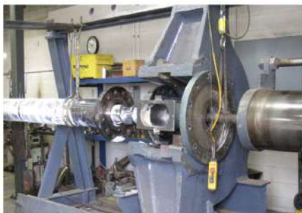
A 25 foot long barrel for plastic extrusion
